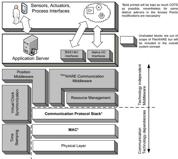
Figure 2. Structure of the FlexWARE system
