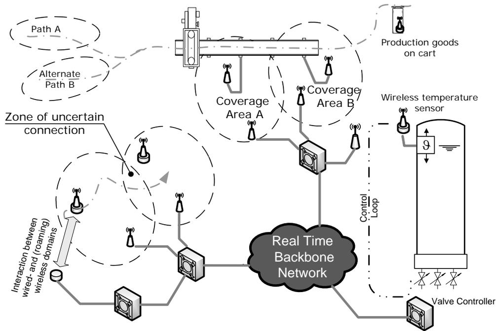
**Figure 1. Proposed system concept, the boxes connected to the Real-Time Network are considered as real-time controllers which are enabled to do the traffic scheduling in both, the wired- and the wireless domain.**
